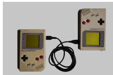
Two Game Boy systems connected with a DMG-04 (link cable). Public domain photo by KoS.
